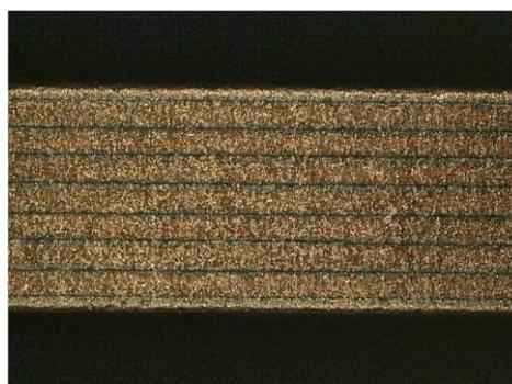
Above images represent cross sections of multi layer SCMC showing the alternative copper and moly stackup. Parts can be cut to simple or complex geometries and plated to meet package and assembly requirements.
