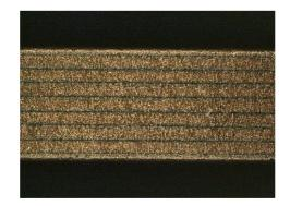
Above images represent cross sections of multi layer SCMC showing the alternative copper and moly stackup. Parts can be cut to simple or complex geometries and plated to meet package and assembly requirements.
